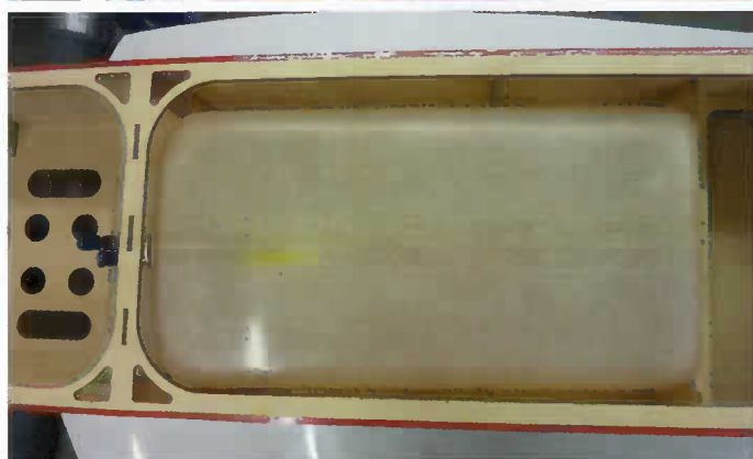
Some sanding is required to fit the fiberglass tank provided with the kit. It's held in place with Velcro tape
