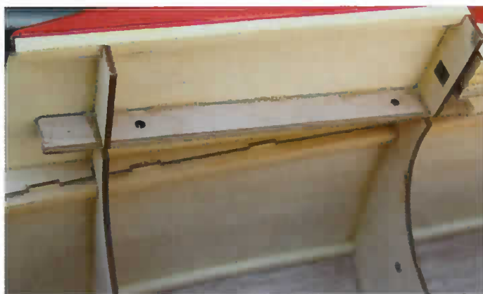
The pre-installed turbine rails have the wrong angle. After removing them, a new set of rails is glued in place
