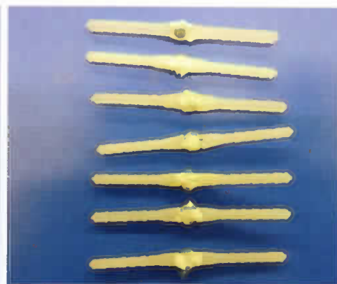
The small pin-hinges proved to be strong enough for the arising forces
