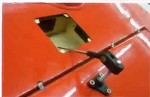
Setting up the controls is quite easy with the provided horns and linkages
