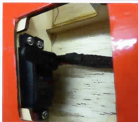
The servos are bolted to the wing-ribs. Dymond DS9999TG all around
