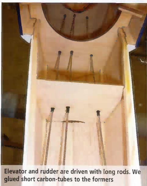
Setting up the controls is quite easy with the provided horns and linkages
